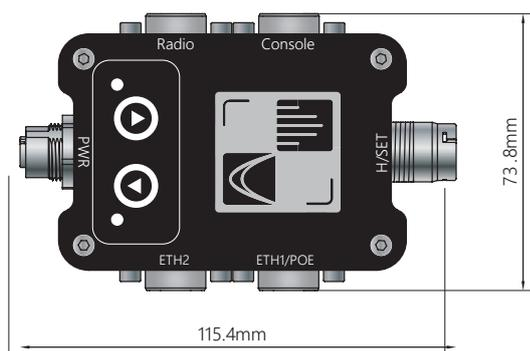
The gateway features connections for one radio, as well as military H-250 handsets. Additionally, network connectivity is through one of two Ethernet ports configured as a 2 port switch. GV1 serves as a data and voice communications hub in mobile or fixed deployments with harsh environments.
